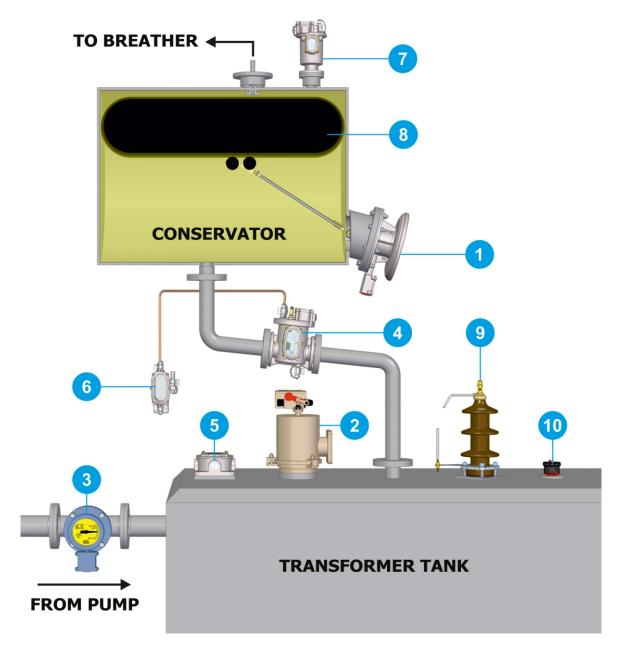
1 Oil Level Indicator 2 Pressure Relief Valve 3 Flow Indicator 4 Buchholz Relay 5 Terminal Box
